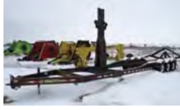
2001 DR21000 - designed to carry 2 headers. (3) 7,000 lb. rubber ride axles, elec. brakes, structural tubing frame.
