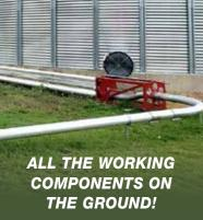
The Ultra-Veyor moves bulk product virtually dust and damage free without the use of heavy augers. Maintenance is performed easily at ground level with simple access to all filters, belts and lubrication points.
